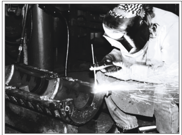
Grooved side-packs of Dresser split repair sleeves prevent gaskets from blowing out of position during installation. Below, a finished sleeve is pressure-tested prior to shipment.
