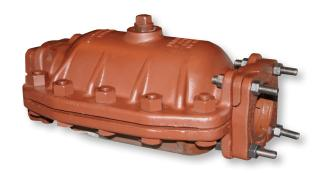
Dresser Style 54 cast split sleeves are designed to completely enclose and repair defective screw collars, plain or butt bell and spigot joints and double-bell circumferential welded joints. Style 54 sleeves can also be used to repair holes and splits up to 8"on steel pipe without service interuptions, and are vented for installation under pressure.
