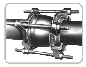
Dresser Style 60-S bell joint clamps are similar to the standard Style 60 clamp, but consist of two spigot rings rather that one spigot and one bell ring. This difference in design is necessary because most stabtype joints, including cast-iron pipe, have a long, tapered bell that has no shoulder for anchoring a bell ring.
