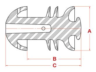
Inhibitor travels through the hollow front cavity and port holes, ultimately leaving a film of protective corrosion inhibitor on the pipe wall.
